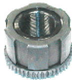
Limited overhead clearance Clamp (SN) Outside Diameter: 1,8 times bolt diameter Height: 1 times bolt diameter
